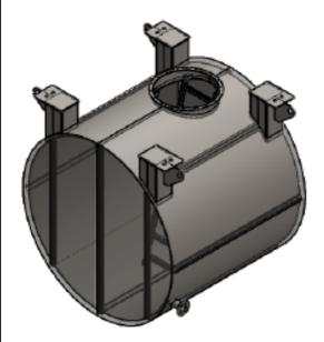
The underground part of the NUP is made of metal. The outer shell is made of steel sheet 4 mm thick, with bottoms at the ends, the inner shell is also made of metal. The thickness of the insulation layer between the inner and outer shells is 50 mm.
